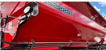
The AS2000 has a stainless steel bin, along the front rear and bottom third, providing longevity.
