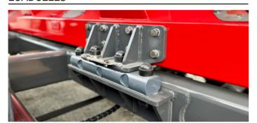
The AS2000 loadcells are standard on all models.
