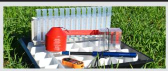
Included as standard to assist with the correct set-up and testing of the rate, flow and distribution pattern of products. The kit includes 13 test trays with dividing inserts, test tubes, bulk density meter, hardness tester, granular sieve, and a windometer.
