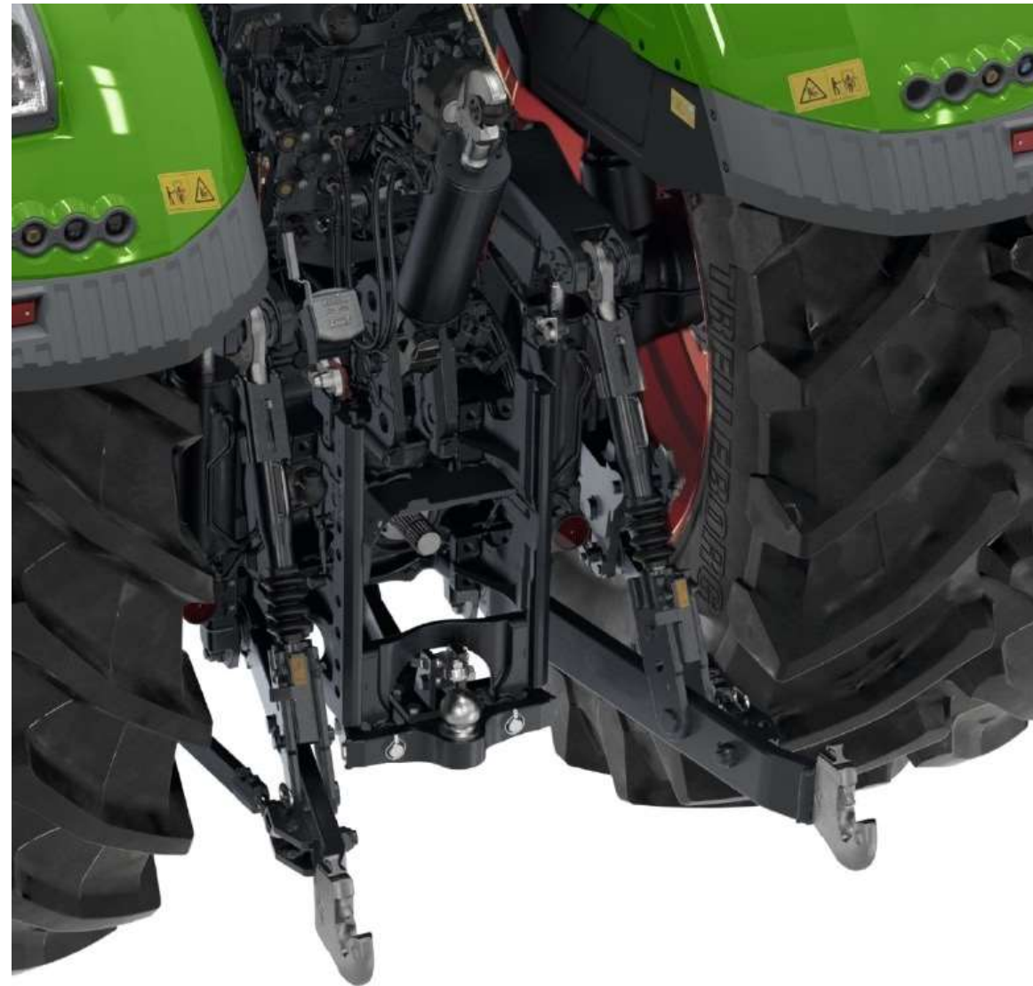
Rear linkage with quick coupler
