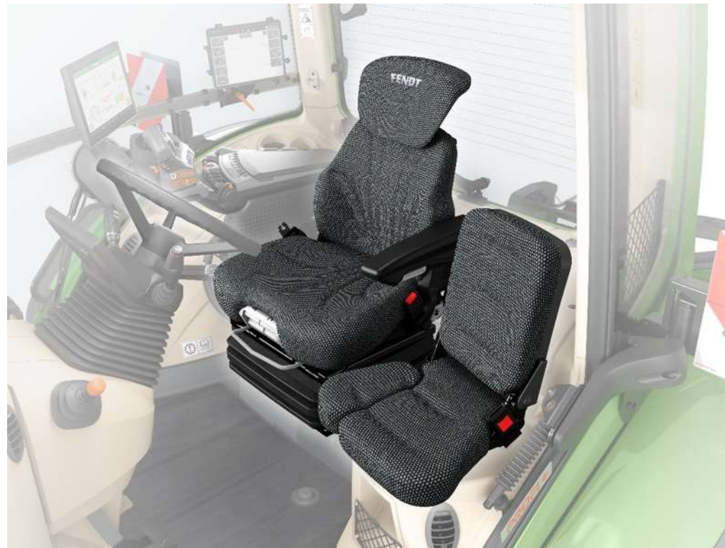
Super comfort seat with air suspension
