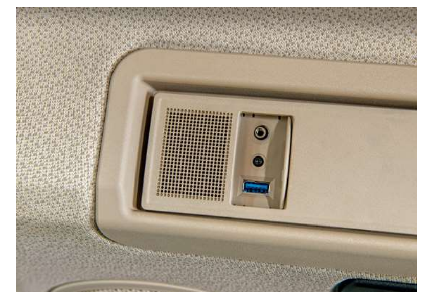
Connection of external audio sources via Bluetooth or cable-based via USB or AUX-IN connection
