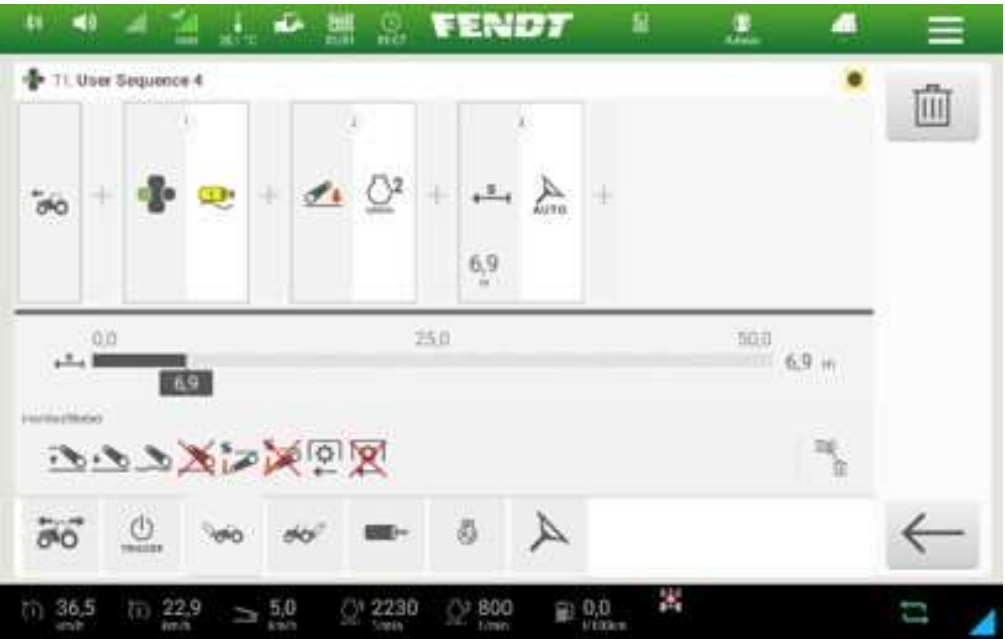
4) Adding the desired function by drag & drop
