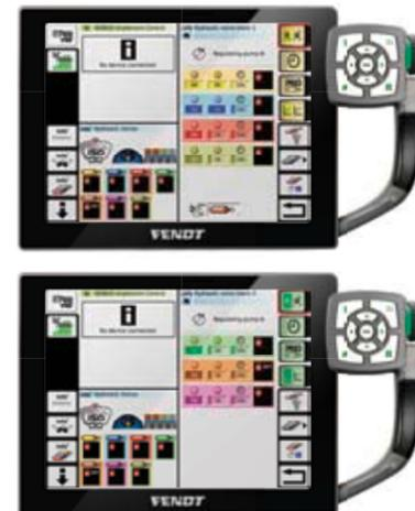
Two valves can be prioritised for the dual-circuit high-capacity hydraulics.
