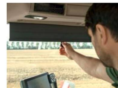
Precise sun protection with one hand movement, also on the right-hand side window.
