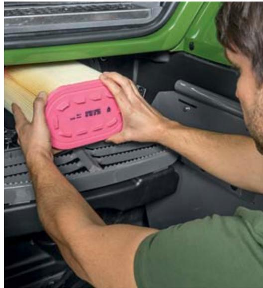
The cab filter is well accessible in the entry area and can be easily cleaned, when necessary.
