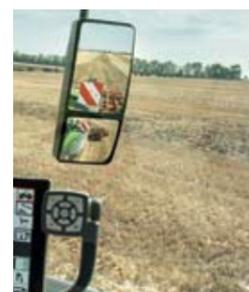
The wide-angle mirrors can be moved freely and extend the viewing angle towards the back.
