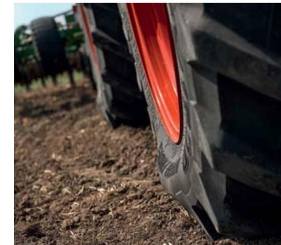
The Grip Assistant recommends the right tyre pressure and ballasting for a defined speed when in Speed Select mode. In Ballast Select mode, the assistant recommends the ideal working speed as well as tyre pressure for a defined ballast.
