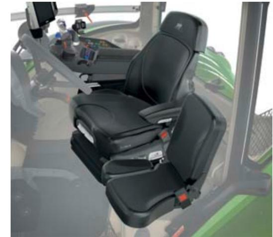
The comfort passenger seat is ergonomically formed and has additional cushioning. Folded down, it turns into a practical table with a clamp for papers.
