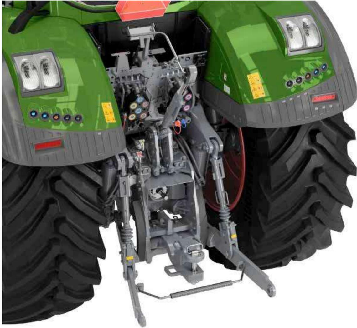
Rear linkage with ball ends and rub blocks
