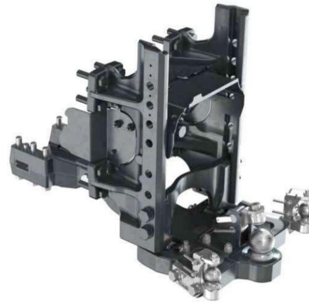
Ball head coupling long (with/without connection points forced steering)
