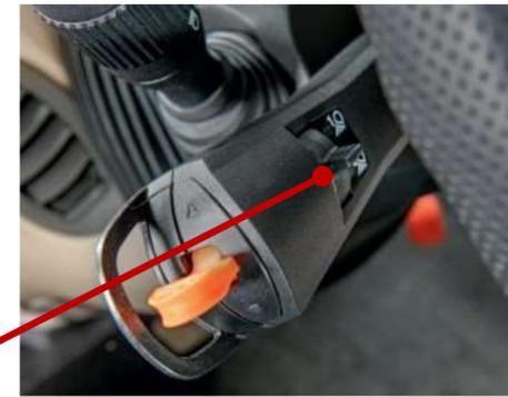
Switch on the reversing lever for activating/ switching between the two stored lighting modes
