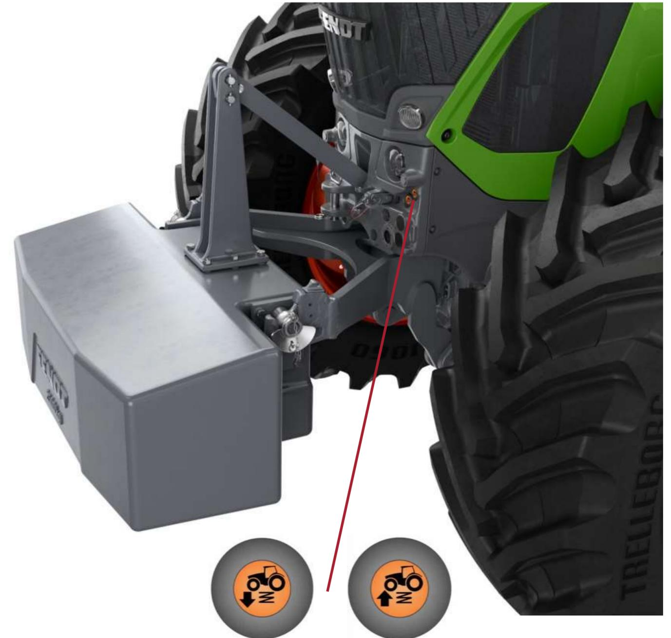
For external operation, there are buttons on the front panel.
