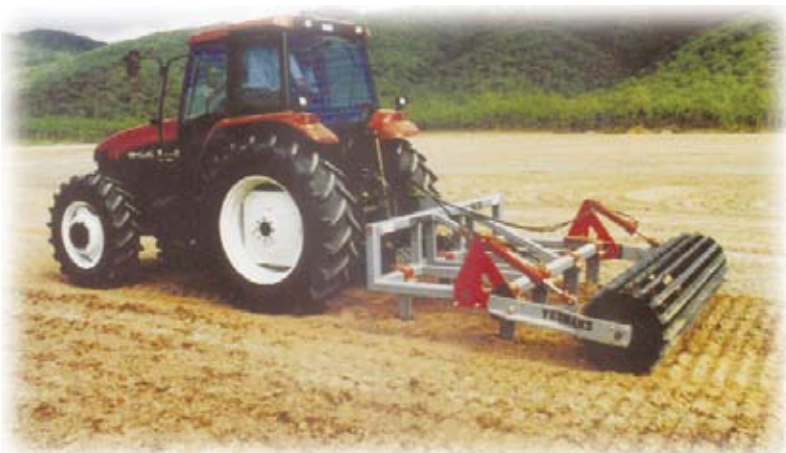
◀ J-9 Fitted with 7 Shanks and a Yeomans Single Crumble Roller
