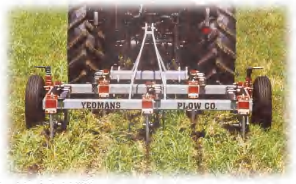
GP39-8 Frame - In Action. The GP39-8 set up with Depth Wheels, five 22" Shanks and 16" Coulters
