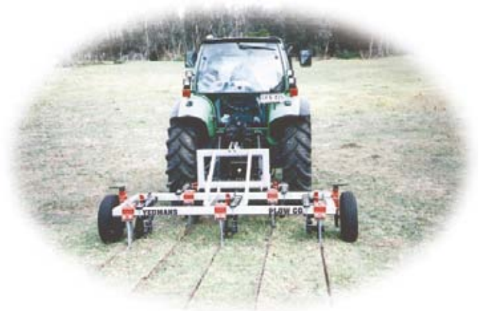
L43-9 with five 26" Shanks and 18" Coulter Happily Subsoiling a Kikuyu Pasture
