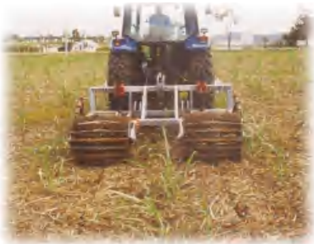
J-9 Fitted with Two Shanks and Yeomans Dual Crumble Rollers
