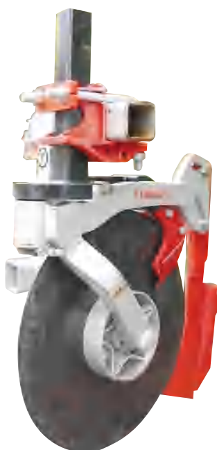
"Jungle Coultter fitted with Adjustable Fertiliser Boot and Scraper Blades."
