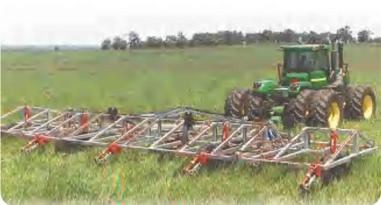
"40" foot (12.2m) Folding Wing Model set up with thirteen Stump Jump Shanks. West of Biloela in central Queensland".
