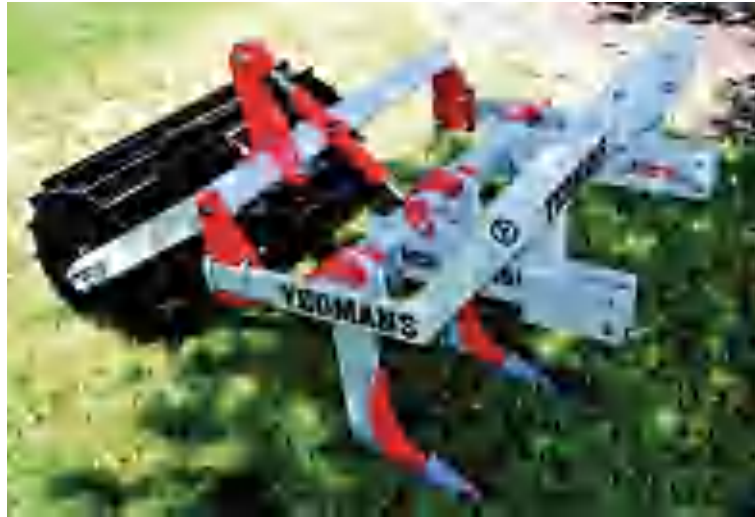
R56 with OCS26C (26") shanks and Crumble Roller
