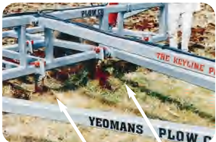
T92-12 with 26" Shanks showing BRAKE-OUT in front of the shanks.
