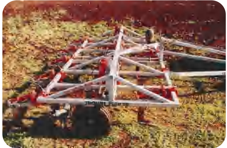
T123Sj-15 with thirteen Stump Jump Shanks at 13" spacing.
