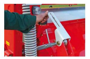
Three-dimensional ground hugging is ensured by the freedom of movement enabled by the cutter bar being suspended in the portal frame.
