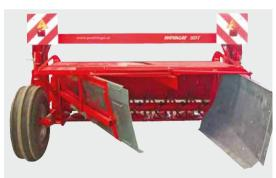
A cost-effective form of swath placement is provided by swath boards, which are adjusted hydraulically.
