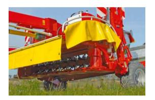
The heart of PÖTTINGER disc mowers is the cutter bar, proven over thousands of cuts in the field. NOVACAT disc mower cutter bars are developed and built at the company's main plant in Grieskirchen – a quality product made in Austria. First-class cutting quality, low drag resistance and strength are the trademarks of these cutter bars. Engineered details guarantee you reliable operation and contribute significantly to an extended service life.
