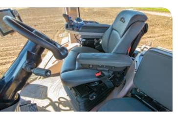
Help lessen operator fatigue with the optional deluxe vibration reduction system (VRS) vented leather seat with semi-active suspension.
